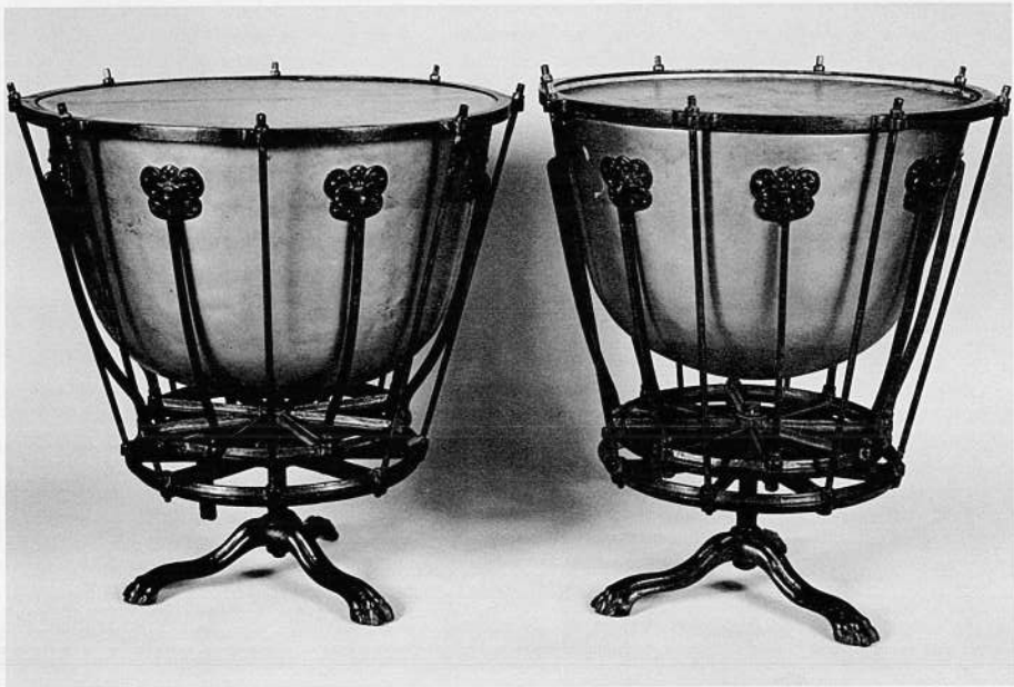
FIGURE 2. Rotary-tuned machine drums of the Stumpff type (German, ca. 1821). Courtesy of the Africana Museum, Johannesburg (Inv. no. KG122).
