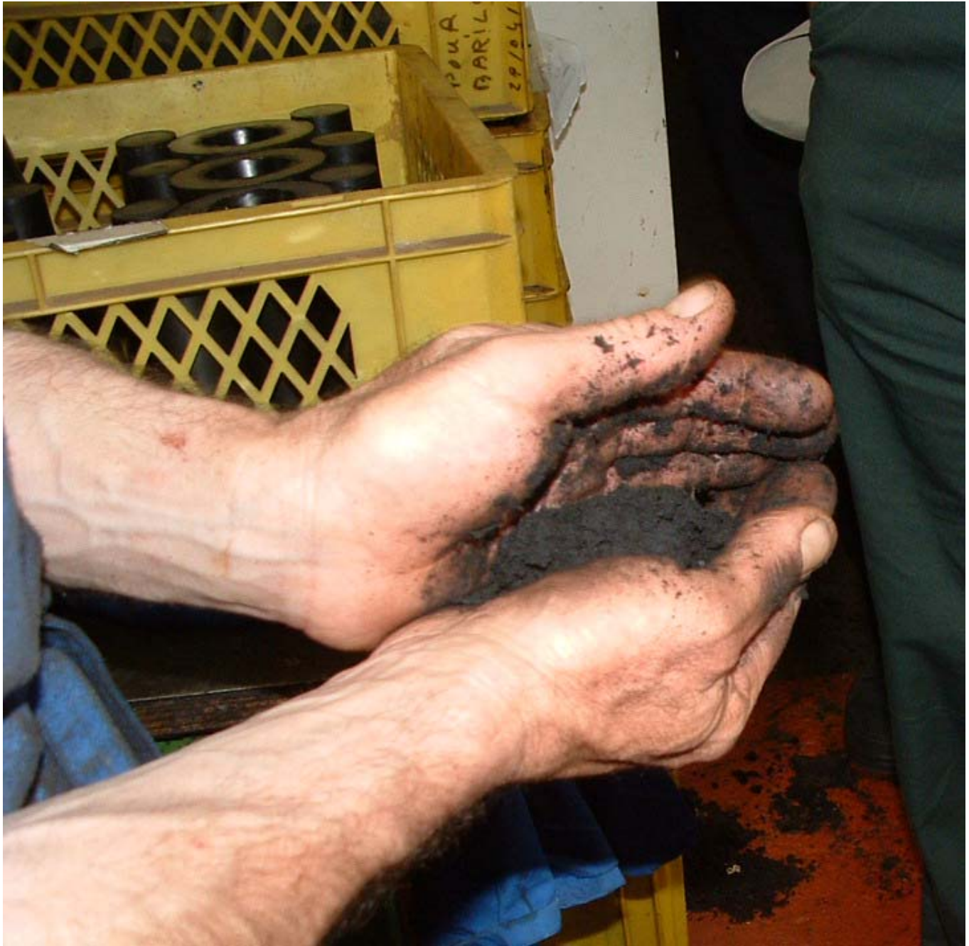
Scrap grenadilla shavings from the Buffet factory floor being prepared for use in the compound used to make 'Green Line' clarinets. Horniman Museum
