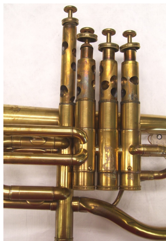
Figure 4.23 Valve section of a contralto saxhorn in B-flat made by Ad. Sax in 1863, with three regular and one ascending valve. Musée de la musique (inventory no. E.744). Photograph by the author.
